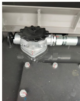
Figure 5-4 Hydraulic return filter
