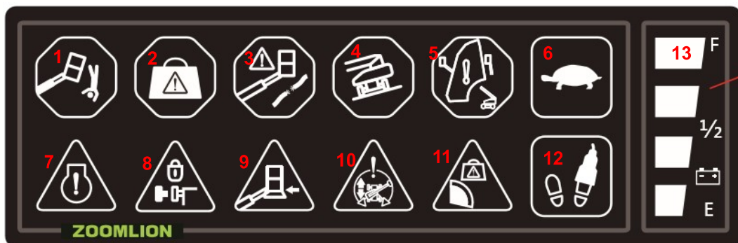
Figure 2-13 Platform Control Indicator Panel
