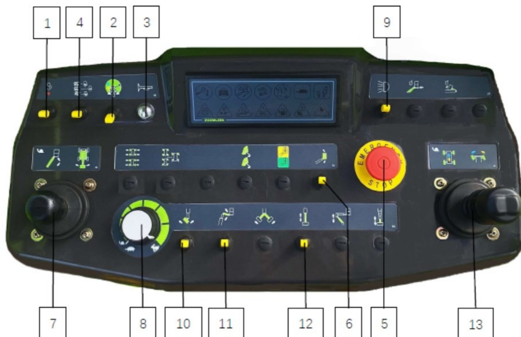
Figure 2-12 Platform Control Panel
