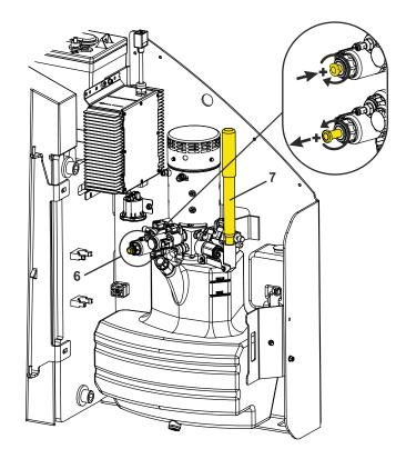
Figure 3-8. Manual Swinging Operating Devices
