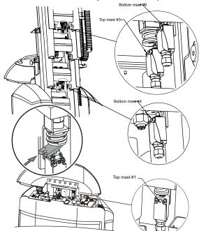
Figure 5-19. Slack/Broken Chain Sensors
