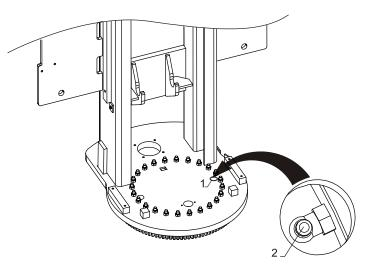
Figure 5-15. Swing Bearing Race Lubrication
