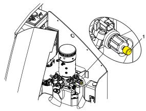
Figure 3-5. Flow Control Valve
