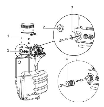
Figure 5-10. Hydraulic Filter Replacement
