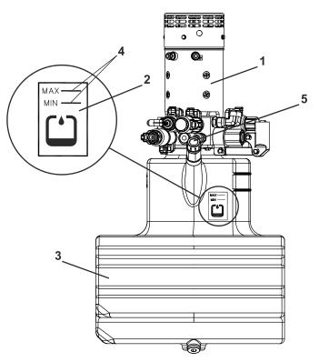
Figure 5-9. Hydraulic Oil Check
