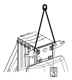
Figure 3-16. Lifting the Machine
