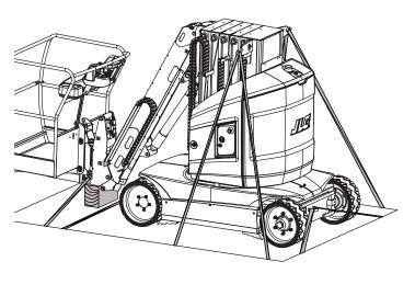
Figure 3-15. Machine Tie-Down
