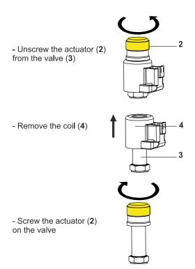
Figure 3-6. Mast Manual Descent Actuator Installation
