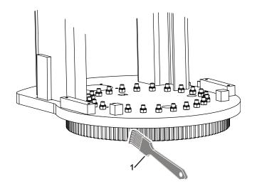
Figure 5-16. Swing Bearing Teeth lubrication
