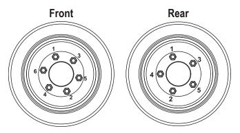
Figure 5-11. Wheel Lug Nut Tightening Sequence
