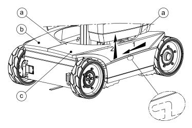
Figure 5-4. Chassis Hood Removal
