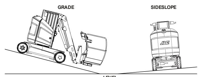
**LEV EL** Figure 3-12. Grade and Side Slope
