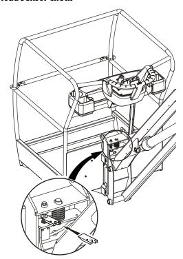
Figure 2-2. Overload Sensor
