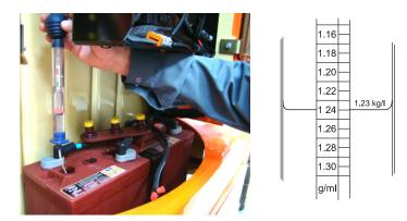
Figure 5-8. Measuring Electrolyte Specific Gravity
